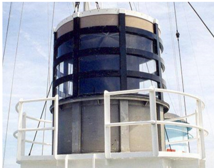
The Type 271 that defeated it, its enclosure giving a distinctive lantern-like appearance (Credit: HMCS Sackville/Jerry Proc).
