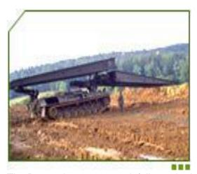
The Beaver is an armoured, fully tracked vehicle built on the chassis of a Leopard Tank. It is a highly mobile, rapidly deployable assault bridge that can be used to span natural and man-made obstacles on the battlefield.
