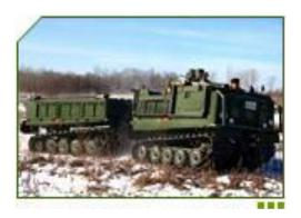
The BV 206 is a special military vehicle designed for use as an all-terrain transport vehicle. It is capable of travel both on and off roads, under almost all conditions and in all climatic extremes. In particular, its large track area allows the vehicle to travel over deep snow and soft ground that would be impassable to almost all other tracked and wheeled vehicles. It is also amphibious, being propelled in the water by its four tracks.
