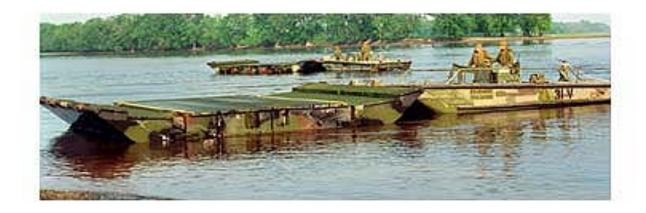
The Medium Floating Bridge (MFB) is used to provide a hasty means of transportation across water obstacles. It can also be configured as a ferry, in which case it is referred to as the Medium Raft (MR). The system is a reverse engineered design of the Russian PMP steel floating fold-bridge and was designed and built in Germany.
