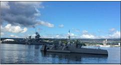
Large Unmanned Surface Vehicle (LUSV) - 200-300 feet length and full load displacement of 1,000-2,000 tons.
