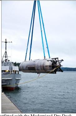
"The LDUUV Phase 2 vehicle will integrate with submarines outfitted with the Modernized Dry Dock Shelter (DDS) and the Payload Handling System (PHS)." I wonder whether there will be any way that LDUUV will be able to connect with Canadian submarines. An universal (or, at least, alliance) coupler? Could be quite the capability enhancement.
