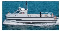
An 11 metres, ship-deployable, workboat configurable (and I take it easily re-configurable) for logistics, diving training and operations, officer training, hydrographic survey, passenger
