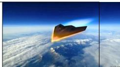
This article suggests: "Missiles that travel at speeds greater than Mach 5 (five times the speed of sound, or about 1.5km per second), have existed for some time. Intercontinental ballistic missiles (icbms) reenter the atmosphere at up to 8km per second. What is different about the hypersonic weapons in the pipeline is that they are designed to sustain such speeds over long distances, manoeuvre as they do so and, in some cases, hit targets with pinpoint accuracy."
