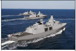
The Type 31e for the Royal Navy is meant to be at the low end of the range of frigate capabilities (greater, by definition, than a corvette). The Babcock proposal, with 100 ship's company and 28 knots speed, has aspects of a low end frigate, but at 5,700 tonnes and 138.7 metres in length, this is not a small ship! Size is not an indicator of a warship's type or capability.
