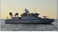
"The Navy specified a 'visual-deterrent' appearance for the new vessel, which the design satisfies with a futuristic and 'menacing' faceted hull profile above the waterline."
