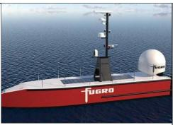
"The first of the 12m SEA-KIT X class USVs ... will feature remotely operated vehicle (ROV) and autonomous underwater vehicle (AUV) launch-and-recovery systems and station-keeping capabilities. The vessel will be used to conduct completely uncrewed ROV pipeline inspections in up to 400m water depth ..."
