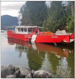
A RUSI(NS) member identified it as a PRV (pollution response vessel) III environmental response barge. A Robert Allan design (RAL are also the designers for the Naval Large Tug project, four tugs of which are being procured for the Queen's Harbour Masters), 14.3 m length and 13.3 tonnes with twin stern drives. There is a smaller PRV II model with twin outboards. "It is believed that there are several tens of PRV across the country."
