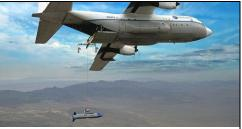
Gremlins program "... experimenting with swarming drones that are designed to be launched and recovered in mid-air." And then re-loaded (and presumably re-charged/fueled).
