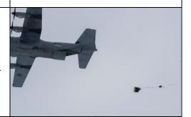
Trenton JRCC CCCOS @JRCCTrentCCCOS 1 Feb tweeted: With a range of over 7000 kms, ability to operate at high and low altitudes, and capacity to carry and drop SAR Techs and equipment, the @RCAF\_ARC's CC-130H Hercules is a great #SAR aircraft for Search and Rescue Region Trenton! @RCAFoperations #ThatOthersMayLive #DYK
