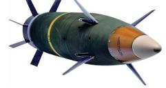
fired, tiny wings spring out of the Excalibur, which then steer it to its destination using GPS data."
