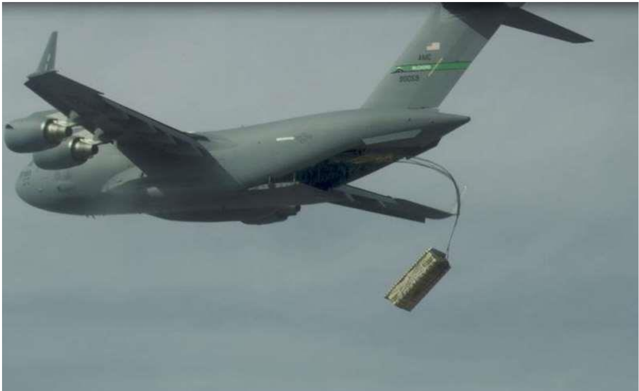
© US Air Force A C-17 drops palletized munitions (simulated JASSMs) during Advanced Battle Management Onramp #2 testing. US Air Force
