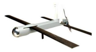
The UAV should weigh less than 36 pounds, and be launched from the aircraft and be able to fly for as long as 45 minutes at cruise speed; fly as fast as 90 knots; and be able to detect a target the size of a submarine.
