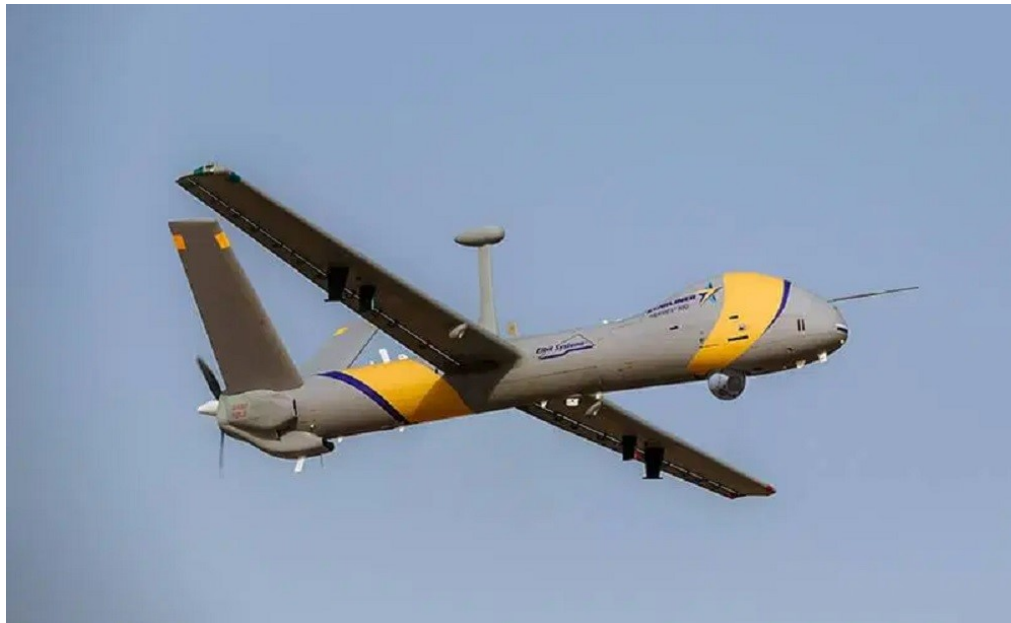
The drone Canada is buying is a civilian version of the Hermes 900 military drone. It has a wingspan of 15 meters, can reach 10,000 meters, can fly for up to 30 hours, with cruise speed at just over 100 km/h. (Elbit Systems)
